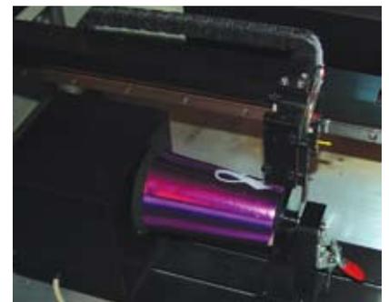
**Figure 3: The GX offers a cylindrical attachment as one of its standard accessories.**
