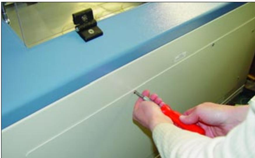
Removing eight screws from the back cover in order to use the pass-through capability is a reminder that this can be dangerous. Precautions should be taken when operating a laser with doors or panels removed.
