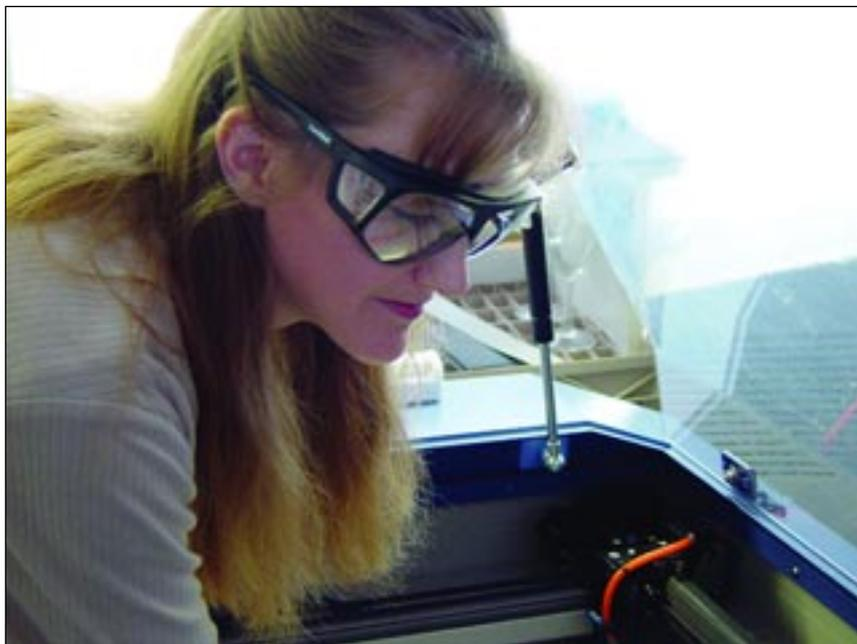
Special LaserShield glasses are a MUST when operating a laser when using the pass-through feature. These special glasses are provided with the laser.
